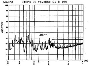
Figure 3 - Emissions Plot for STP System C
