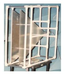
Figure 1: TEM "Time Domain" Antenna
