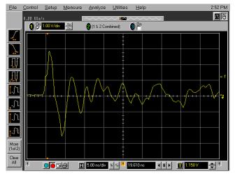
Figure 4: Field Strength Resulting From Disk Drive Insertion
