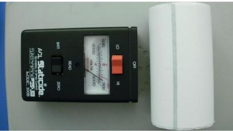
Figure 1. Measuring the Approximate Charge Voltage on the Print Media
