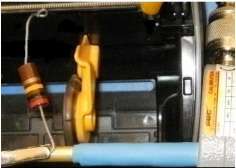
Figure 5. Applying a Discharge to the Printhead
